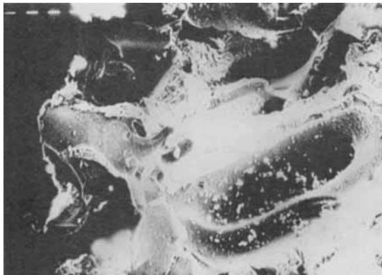
Fig. 2. SEM view of the foam sample from 80% PS and 20% PMMA X32.
